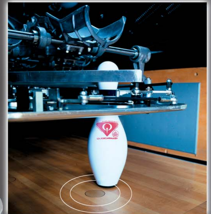
The 90XLi out of range pin area is 1.44 times greater than competing machines, so manual respots are rare.
